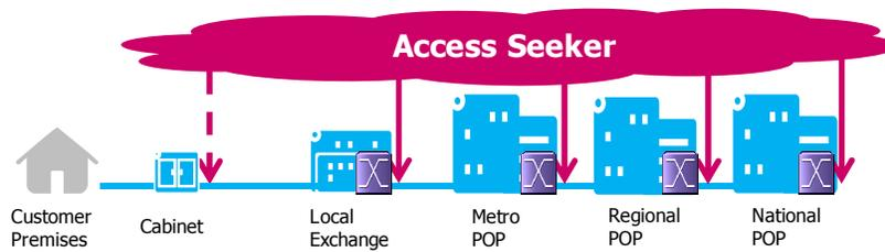
*Figure 2: Next-Generation Bitstream (Ethernet-based)*
