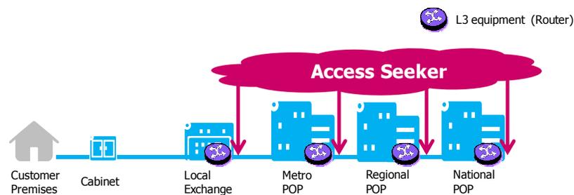
*Figure 3: IP-level Bitstream*
