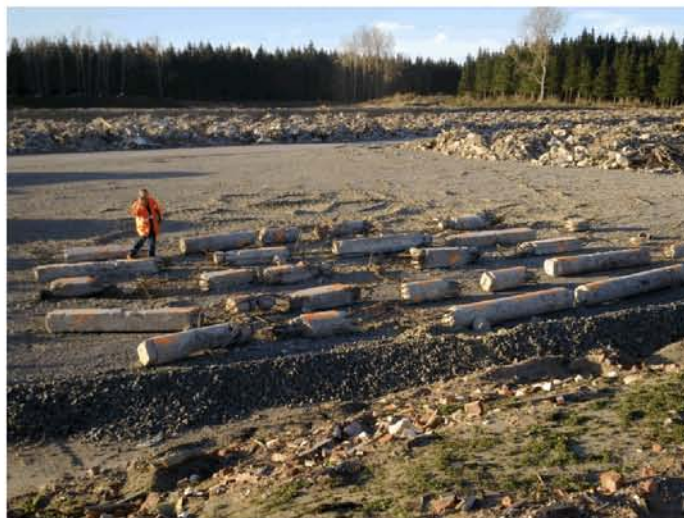
Figure 46 - CTV Building columns extracted for examination and testing from the Burwood debris field.
