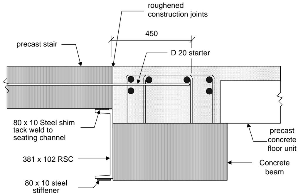
Figure 39 - Typical upper landing support detail.
