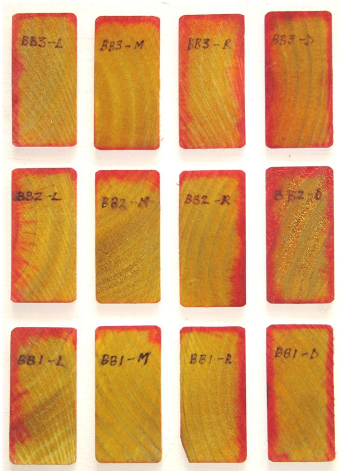
Figure 13 – Penetration of boron in ‘double coat brush-on’ treated units, BB1 at the bottom, through to unit BB3 at the top. Samples, from the left side, are left stud, middle stud, right stud and nog. There was generally 5-10mm penetration only from the surfaces that the preservative was brushed on to.
