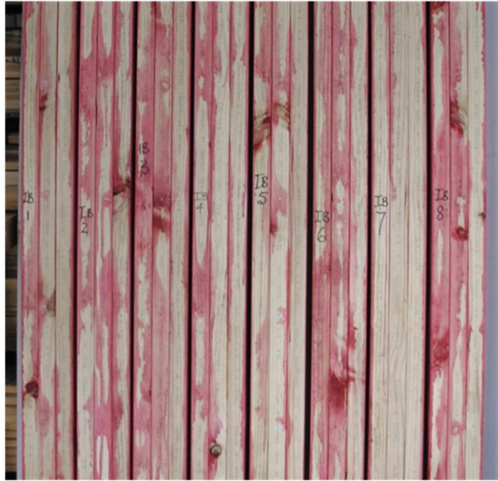
Figure 9 – Boron ‘brush on plus injections between the studs’ units with the plaster board removed (showing the edges of studs originally attached to plasterboard) starting with unit IB1 on the left through to unit IB8 on the right. The preservative had penetrated from the injection holes through to the plasterboard in irregular patches but there was little penetration from the brushed surfaces.
