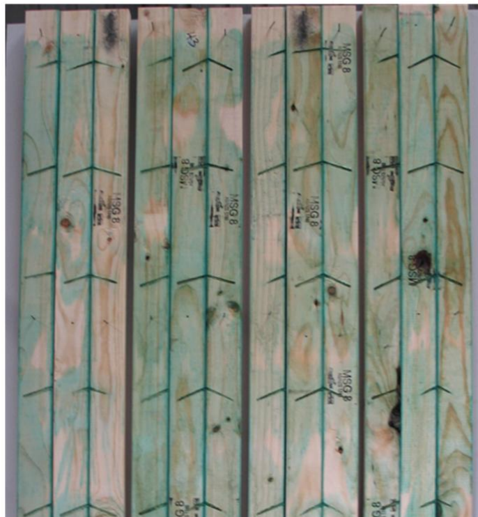
Figure 12 – The concealed faces of ‘brush on plus injections between the studs’ copper naphthenate treated studs (after dismantle), unit IC1 on the left through to unit IC4 on the right. Preservative had spread out from the injection holes.
