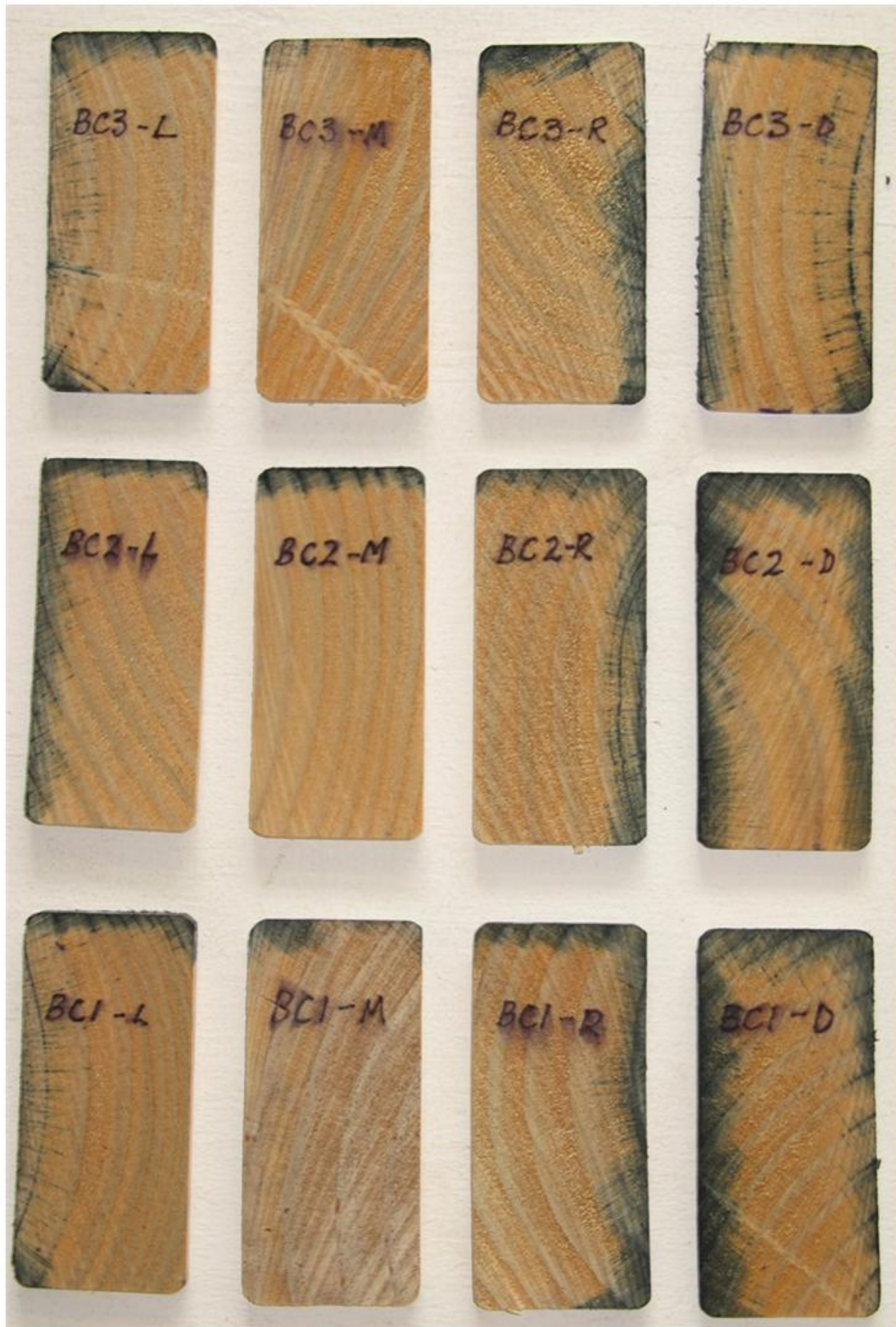
Figure 14 – Penetration of copper in ‘double coat brush-on’ treated units, BC1 at the bottom, through to unit BC3 at the top. Samples, from the left side, are left stud, middle stud, right stud and nog. Penetration was variable from the exposed surfaces and was largely via the medullary rays i.e., at right angles to the growth
