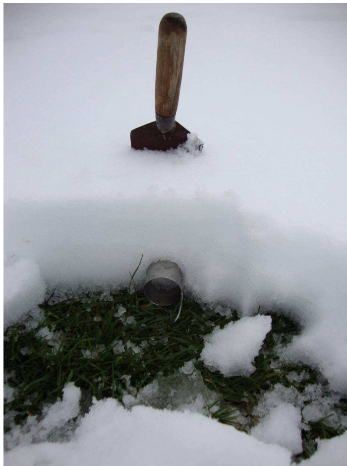
Figure 4: Snow density is measured by excavating a profile wall in the snowpack and then inserting the density cutter at different elevations in the profile. The cutter is then carefully removed and placed on a calibrated scale (Photo: Andrew Willsman).
