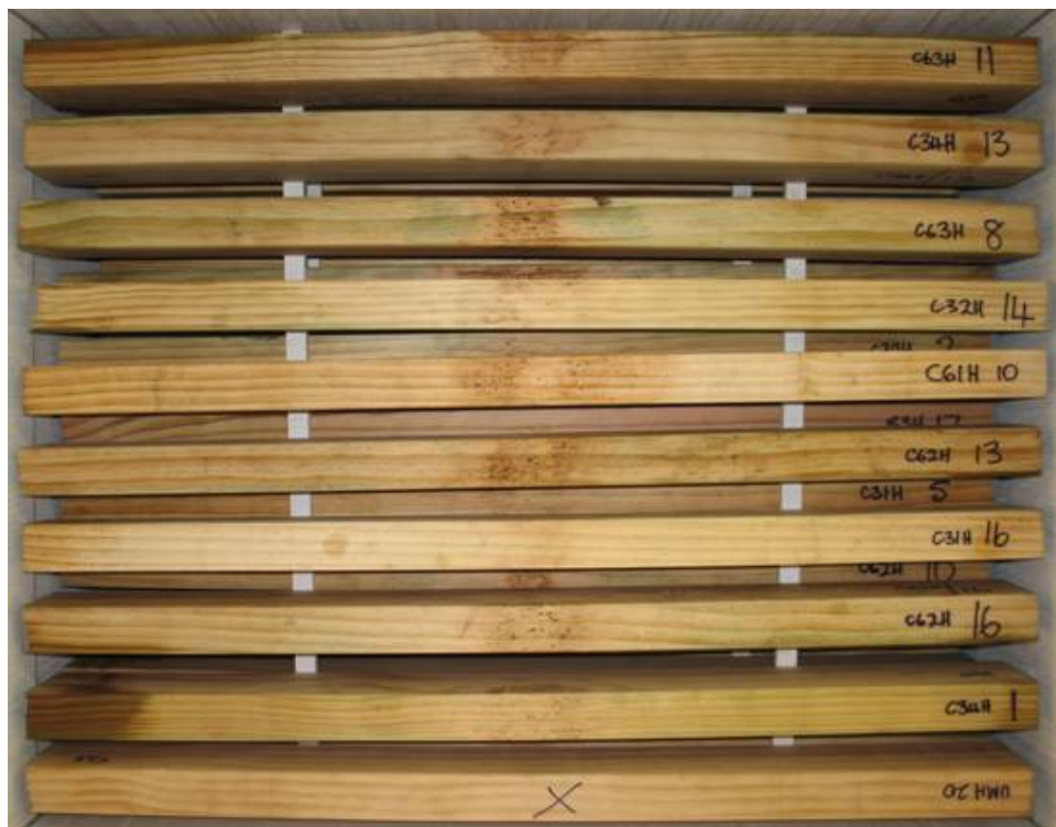
Figure 2 – Copper naphthenate treated HMC samples in tank 2, layer 1 (5 th from top), after 32 weeks exposure. Very little obvious difference since the 16-week assessment.
