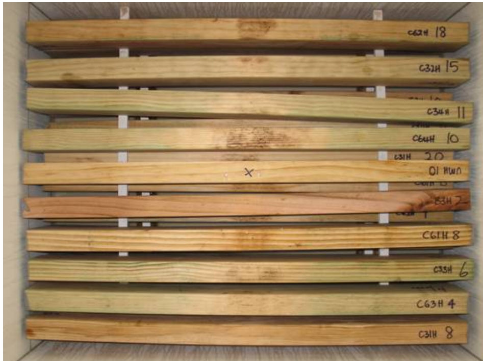
Figure 1 – Copper naphthenate treated HMC samples in tank 4, layer 2 (2 nd from bottom), after 16 weeks exposure. The colour of the preservative had faded slightly and initial decay areas were still visible.
