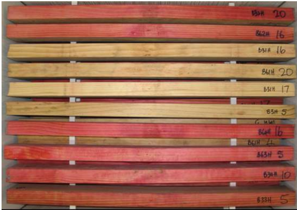
Figure 3 – HMC boron treated samples in tank 6, layer 4 (3 rd from top), after 16 weeks exposure. There few obvious changes in the samples and areas of decay from the original feeder blocks were still visible.
