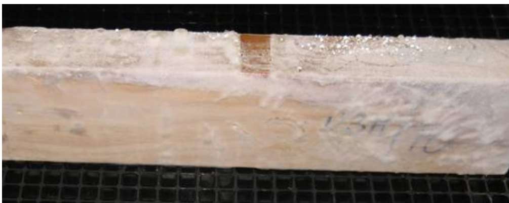
Figure 10 – Untreated sample U3H/10, after 32 weeks exposure. Decay mycelium had spread over most of the surface but the wood was still relatively sound and deflection had only increased by 16%.
