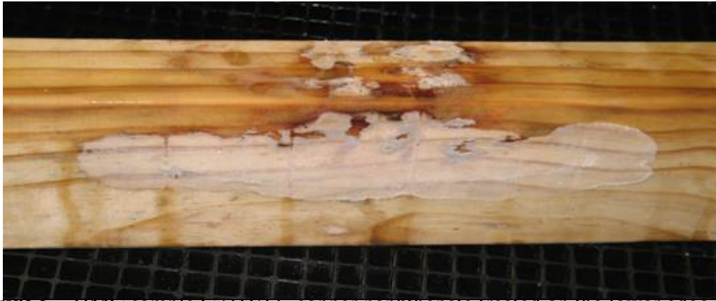
Figure 5 – HMC sample C31H/11, copper naphthenate treated on the lower edge, after 16 weeks exposure. Decay mycelium spreading from the original infected area but there was no obvious softening of the wood underneath.
