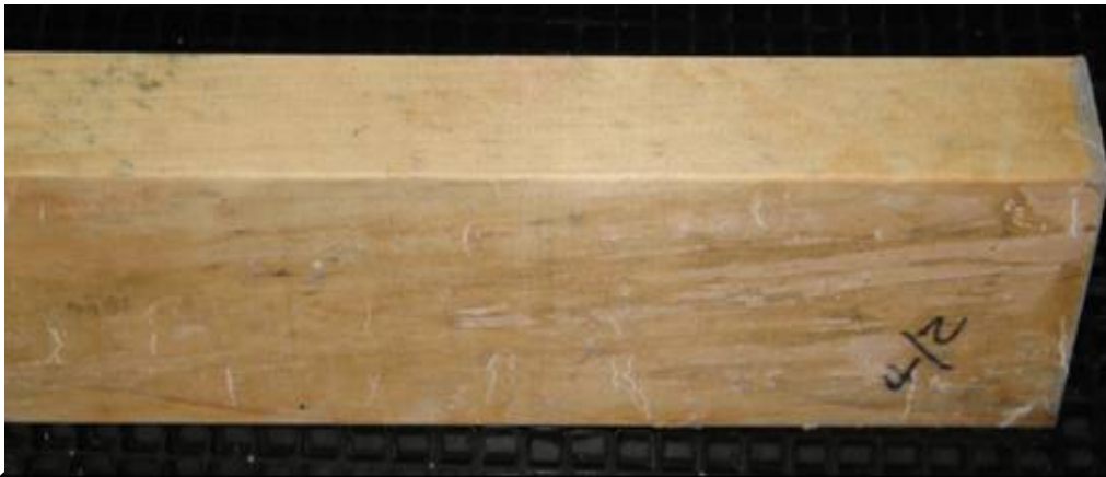
Figure 6 – Untreated sample (not pre-decayed) UMH/15, after 16 weeks exposure. Fine mycelium and pale discoloration developing at one end.
