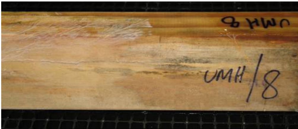
Figure 9 – Untreated sample (not pre-decayed) UMH/8, after 16 weeks exposure. Decay mycelium and pale discolouration at one end appeared to have come from outside contamination.
