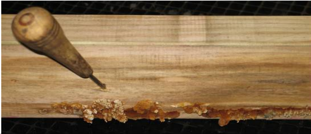
Figure 14 – LMC sample C62L/6, after 52 weeks exposure. Decay fruiting bodies and moderate decay between the treated edges. This sample was in the bottom layer of the LMC stack and deflection had increased by 30%.
