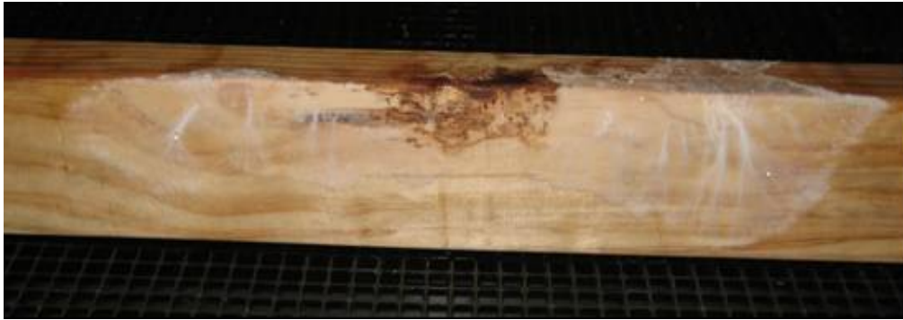
Figure 8 – Untreated sample U3H/10, after 16 weeks exposure. Decay mycelium was developing over an extensive area around the original infection.
