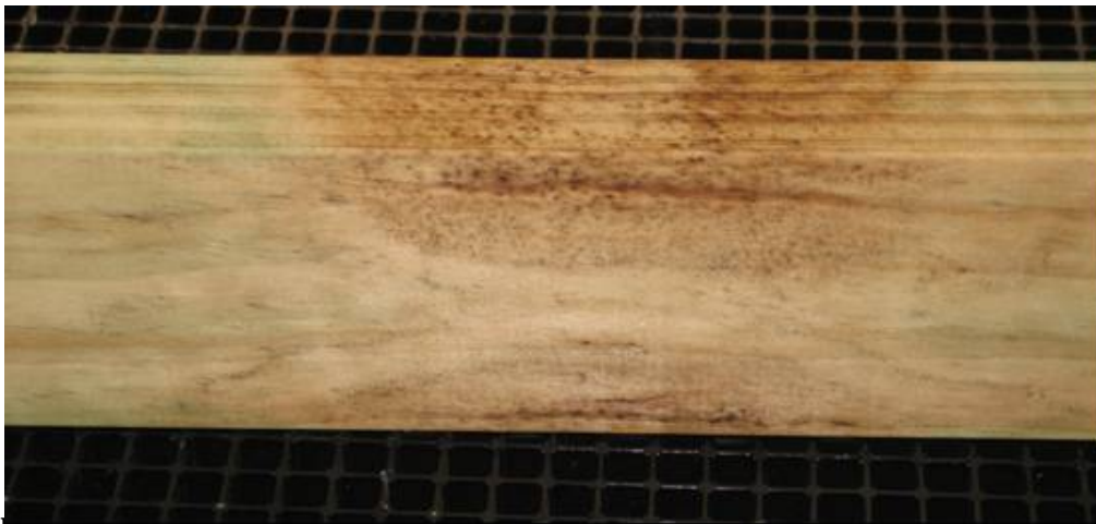
Figure 12 – HMC sample C64H/1, after 32 weeks exposure. Decay was well established on both edges before treatment but has not increased since the sample was treated on all four sides.
