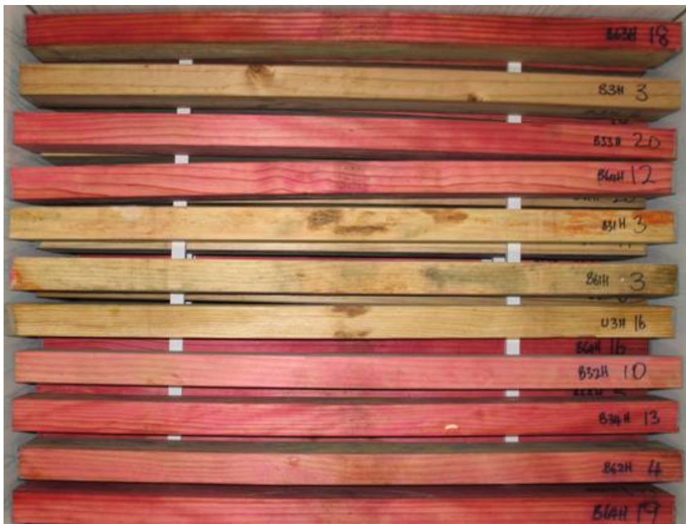
Figure 4 – HMC boron treated samples in tank 6, layer 5 (2 nd from top), after 32 weeks exposure. There was more mould and a patch of decay mycelium on the samples treated on one edge in the centre of the tank but few other obvious changes since the 16 week assessment.
