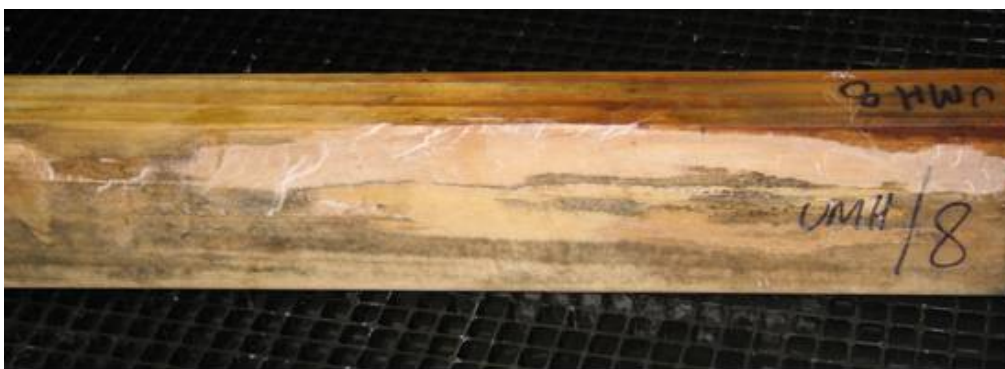
Figure 13 – Untreated sample (not pre-decayed) UMH/8, after 32 weeks exposure. Decay now lightly established at one end but deflection largely unchanged.
