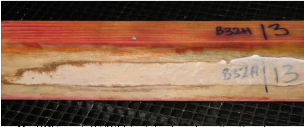
Figure 11 – HMC sample B32H/13, treated on two edges, after 32 weeks exposure. Decay mycelium spreading on the faces between the treated edges. Light – moderate decay was present but deflection had increased by only 5%.
