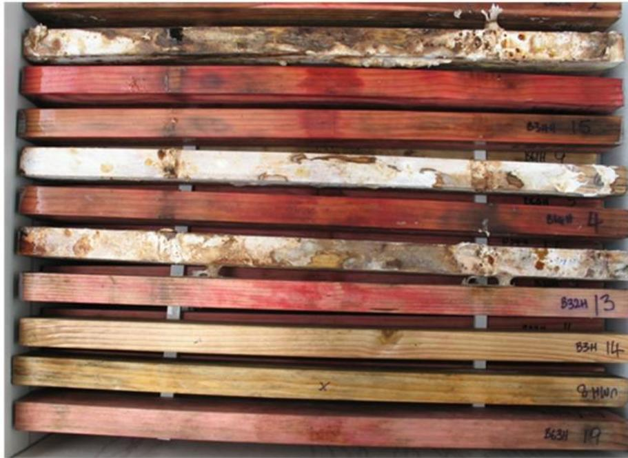
**Figure 11** – HMC boron treated samples in tank 4, layer 6 (top), after 84 weeks exposure. Decay mycelium was beginning to degenerate but there were some patches of fresh growth.
