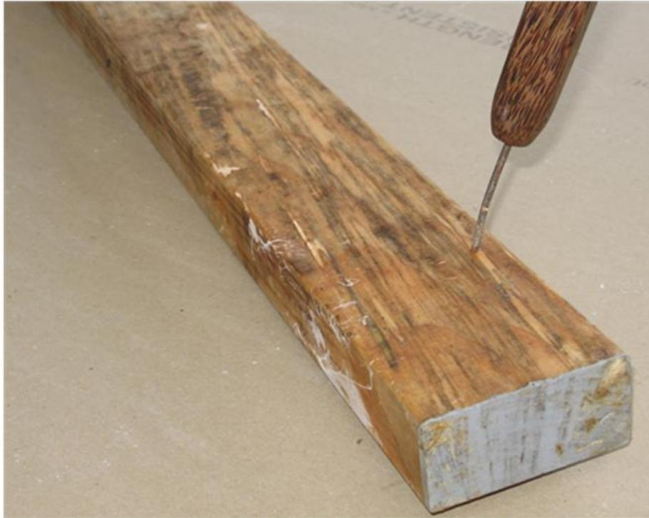
**Figure 20** – Untreated sample UMH/15 (not pre-infected), after 108 weeks exposure. Decay mycelium and small decay pockets, probably from outside contamination, developing along the length of the sample.
