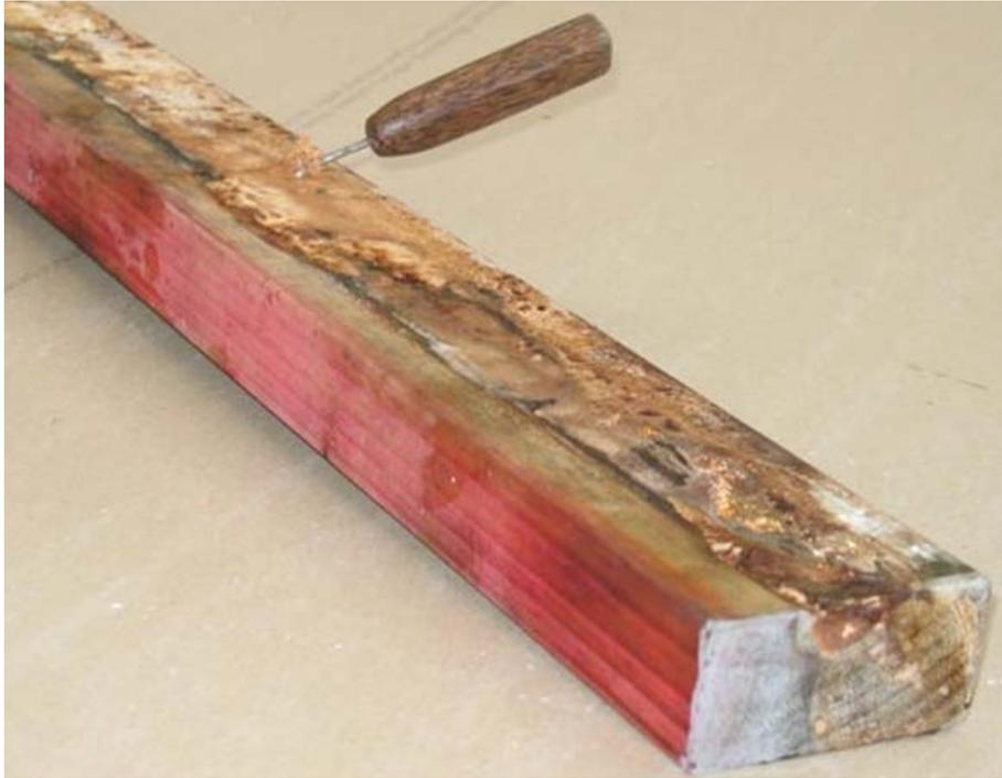
**Figure 18** – HMC sample B61H/12, treated with boron on one edge, after 108 weeks exposure. Extensive mycelium and severe decay on the untreated surfaces away from the boron treated edge.
