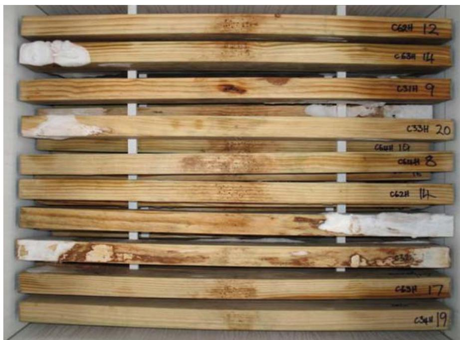
**Figure 10** – Copper naphthenate treated HMC samples in tank 1, layer 4 (3<sup>rd</sup> from top), after 108 weeks exposure. Samples were drier than in the top layer but there were fresh mycelium patches on the treated surfaces of the 2<sup>nd</sup> and 4<sup>th</sup> samples from the top and the 4<sup>th</sup> sample from the bottom in this photo.
