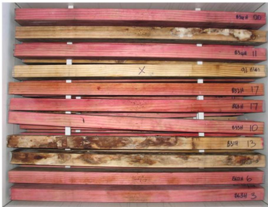
**Figure 14** – HMC boron treated samples in tank 4, layer 4 (3<sup>rd</sup> from top), after 108 weeks exposure. There was no fresh mycelium on the samples. The 3<sup>rd</sup> from the bottom in this photo was untreated and failed at the 108-week assessment. The other samples with mycelium on them were treated on the lower edge only.
