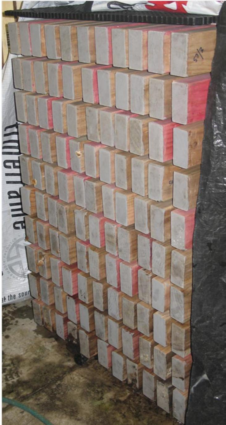
**Figure 15** – LMC sample stack in the controlled condition room after 107 weeks exposure. There were decay fruiting bodies on the ends of four samples in the bottom row (layer 1) and on a few other samples in the stack up to layer 7. These were either untreated control samples or samples that had been treated on two edges only.
