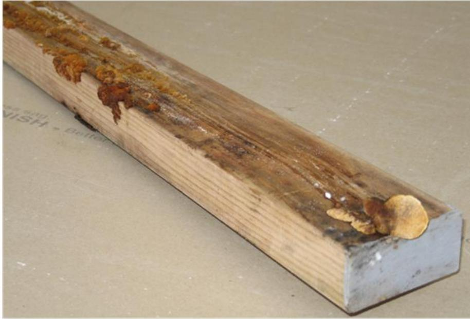
**Figure 22** – LMC sample C32L/3, copper naphthenate treated on two edges, after 107 weeks exposure. There was severe decay and associated fruiting bodies on both faces, spreading onto the treated edges.
