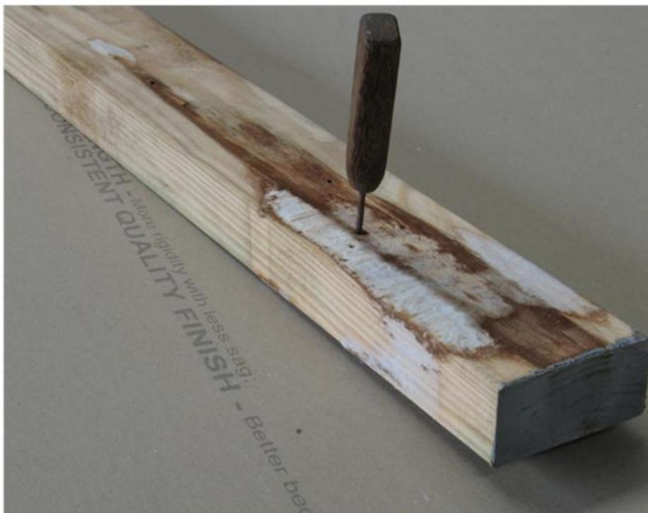
**Figure 17** – HMC sample C64H/16, treated with copper naphthenate on four sides, after 108 weeks exposure. Moderate decay has spread and broken through to the surface from the original decay feeder block infection site.
