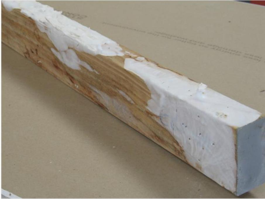
**Figure 16** – HMC sample C62H/8, copper naphthenate treated on two edges, after 108 weeks exposure. There was extensive mycelium developing on all surfaces. Decay was mainly on the untreated faces and on the edge where the original decay feeder block had been attached. here was only minor decay under the mycelium on the treated edges.
