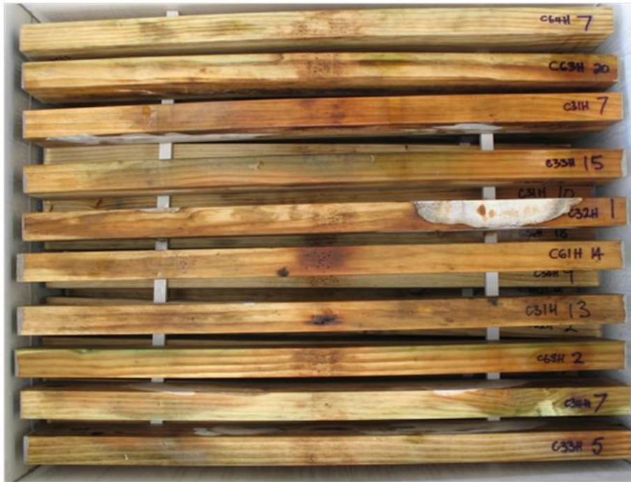
**Figure 7** – Copper naphthenate treated HMC samples in tank 1, layer 6 (top), after 84 weeks exposure. Patches of active, fresh decay mycelium on several samples spreading on to the treated edge of sample B32H1 near the centre of the tank.
