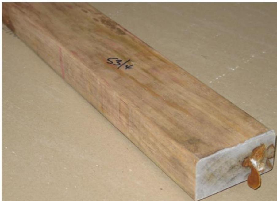
**Figure 21**– LMC sample C64L/7, treated with copper naphthenate on four sides, after 107 weeks exposure. A decay fungi fruiting body on the end was the only indication that there was an internal decay pocket extending out from the original decay feeder block infection.
