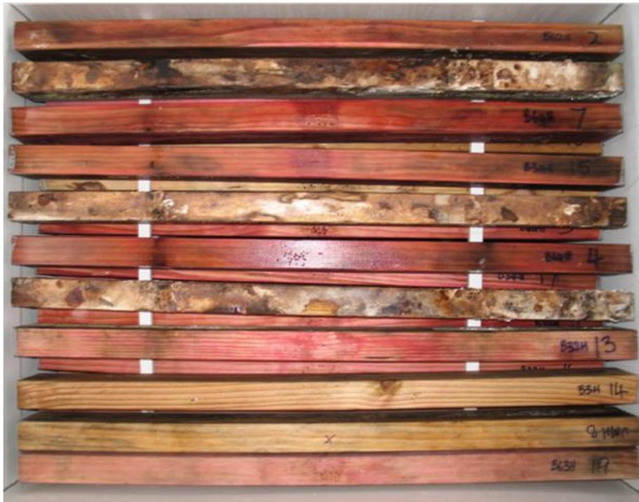
**Figure 12** – HMC boron treated samples in tank 4, layer 6 (top), after 108 weeks exposure. Decay mycelium appeared to be less active than in the tanks containing the copper naphthenate treated samples. The samples with severe mycelium on them were all treated on the lower edge only.
