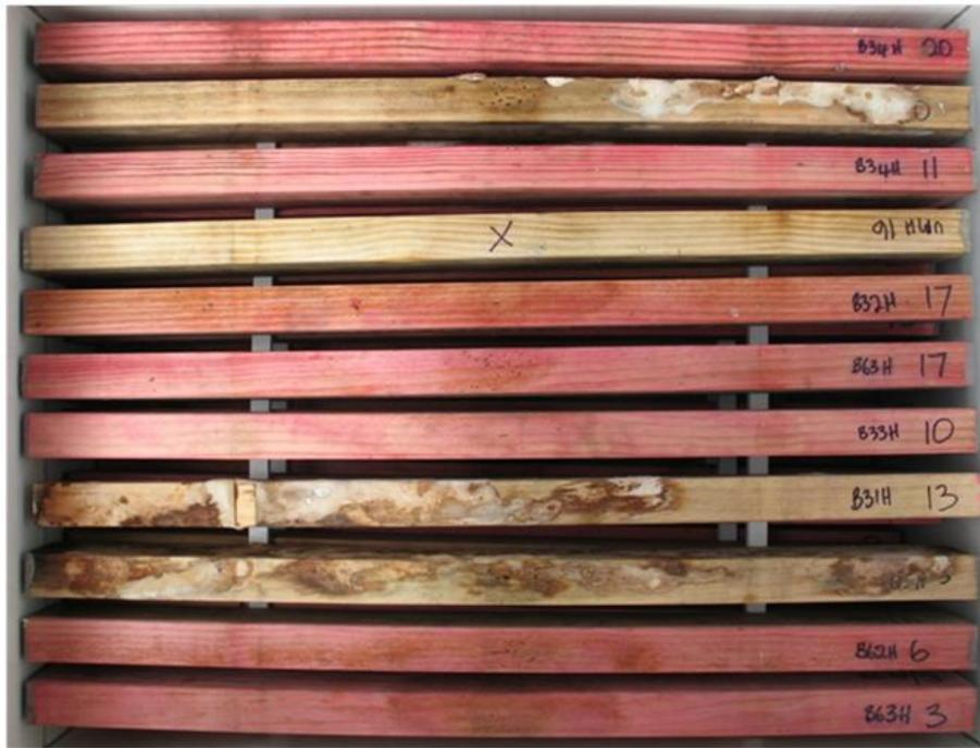
**Figure 13** – HMC boron treated samples in tank 4, layer 4 (3<sup>rd</sup> from top), after 84 weeks exposure. The samples were relatively dry but there was occasional fresh mycelium on the samples and patches of degenerating mycelium.
