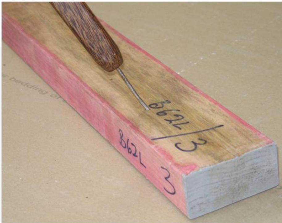
**Figure 23**– LMC sample B62L/3, boron treated on two edges, after 107 weeks exposure. There was light-moderate decay spreading internally towards one end from the original decay feeder block infection area.
