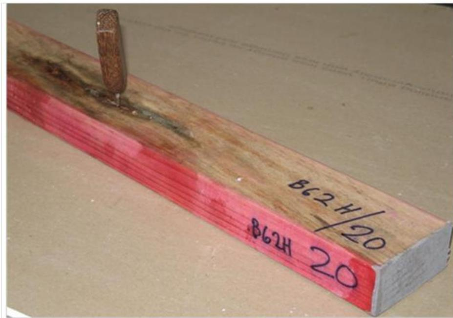
**Figure 19** – HMC sample B62H/20, treated with boron on two edges, after 108 weeks exposure. No active decay mycelium on the surface but moderate decay in the centre away from the boron treated edges.
