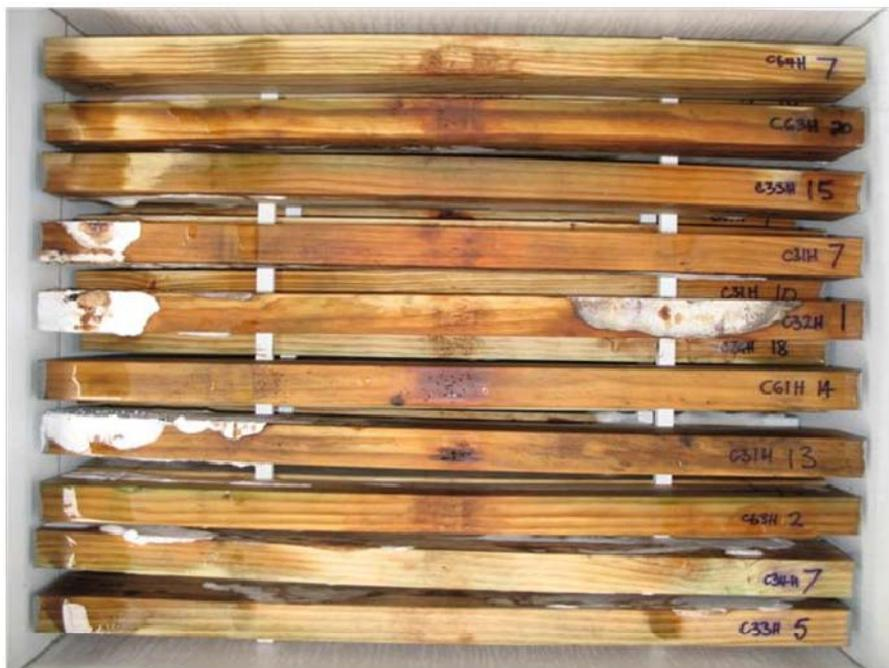
**Figure 8** – Copper naphthenate treated HMC samples in tank 1, layer 6 (top), after 108 weeks exposure. Patches of active, fresh decay mycelium on many of the samples. Active mycelium is visible on the treated surfaces of the two samples at the bottom and the 5<sup>th</sup> sample from the top in this photo.
