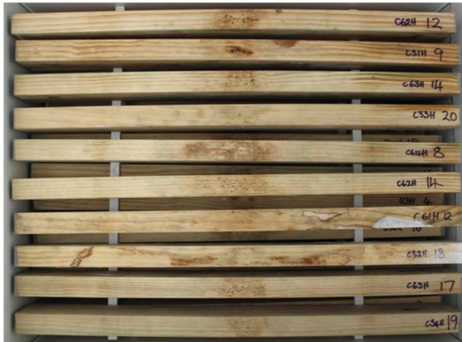
**Figure 9** – Copper naphthenate treated HMC samples in tank 1, layer 4 (3<sup>rd</sup> from top), after 84 weeks exposure. Samples were relatively dry but there was fresh mycelium on the treated edge of sample C32H/18.
