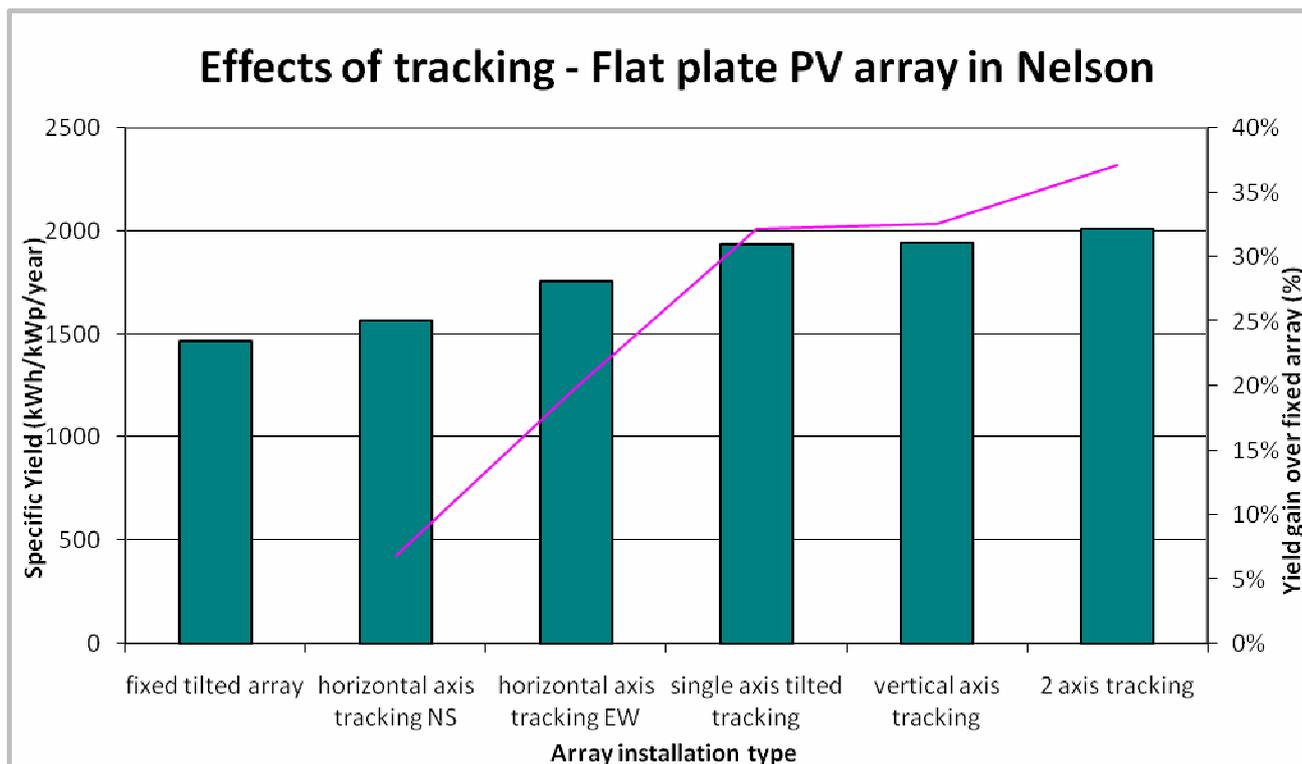
**Figure 2.2: Specific yield gain as a result of array tracking (based on PVsyst simulations for Nelson). The pink line shows the percentage gain over a fixed array.**
