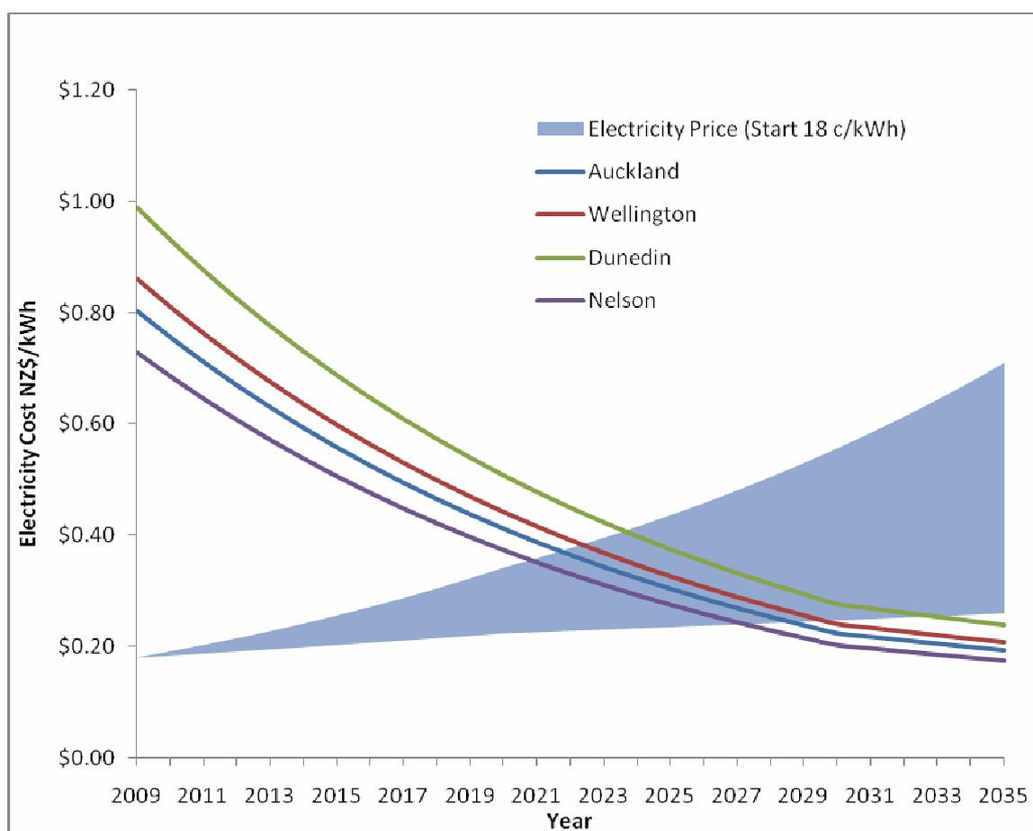
**Figure 8.3: Commercial PV Projections.** Electricity price projections (2008 NZ\$), based on increases in the range 2% then 1% and 6% then 5% per annum, and PV electricity price projections for commercial roof-top systems using multi-crystalline PV to begin with and progressing over time to include 2nd and 3rd generation technologies. For assumptions, see Appendix 2.
