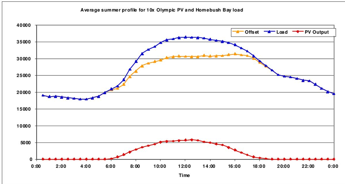
**Figure 4.2: Average Summer Load Profile for the Homebush Bay substation showing the impact of 10x the current Olympic Park installed PV capacity (Watt, 2006)**
