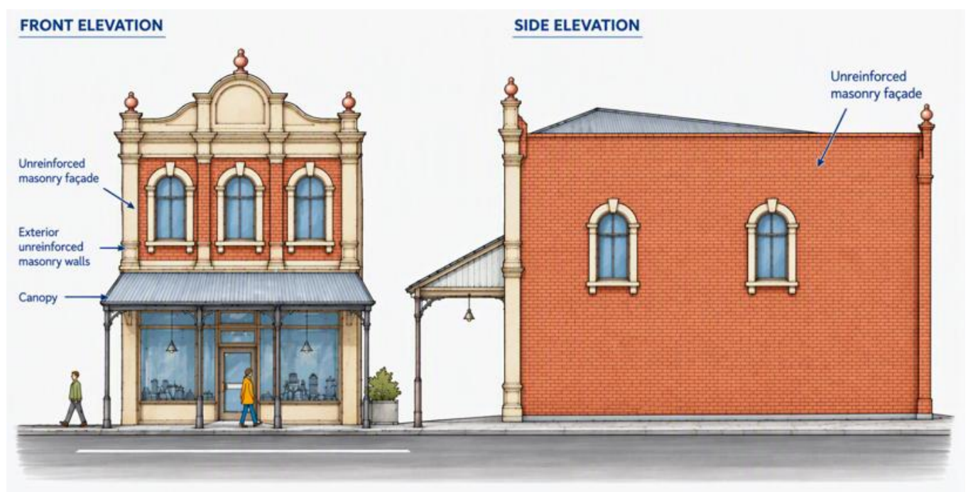
Figure 2: A typical Category A type building
