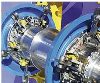
The pig's translational and rotational movements are measured with the help of accelerometers and gyroscopes, which are the main components of this inertial system. After compensating for the earth's rotation, gravitation and other forces, it determines orientations and velocities in X, Y and Z directions. By correlating the inertial system results with the data from dippers and odometer information, the pig computes the exact orientation and position of the pipeline in three dimensions.
