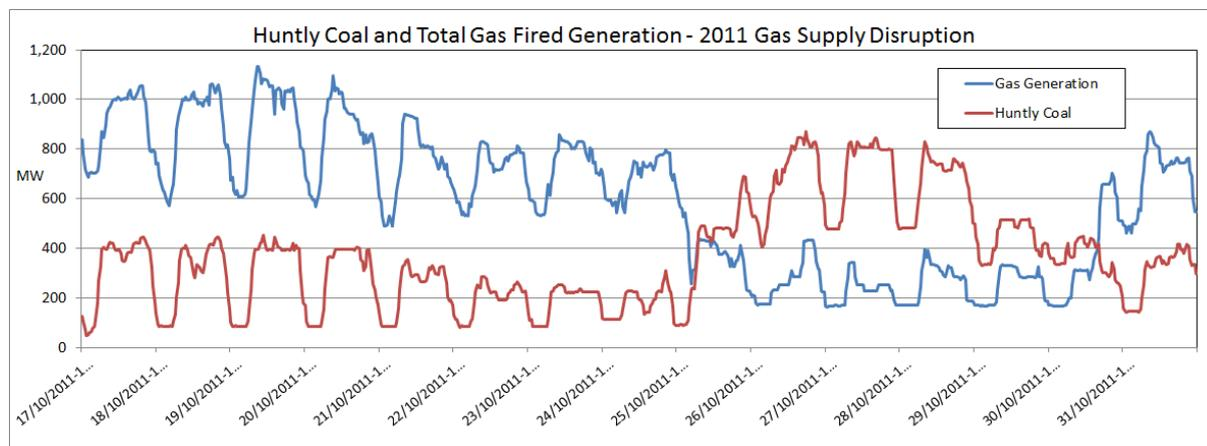
**Figure 13: - Gas and coal generation total, showing the rapid changeover to coal fired generation at Huntly, and the start-ups of the 3<sup>rd</sup> and 4<sup>th</sup> units**
