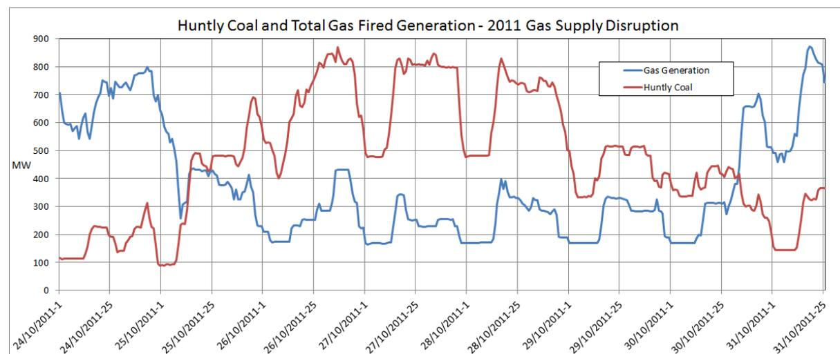
Huntly unit 4 started soon after the curtailment instruction as it was hot following a shutdown at 11:30 pm just prior to the curtailment notice being issued. Huntly’s remaining coal fired units 1 and 2 were cold resulting in long start up times. Huntly units started at the following times:
