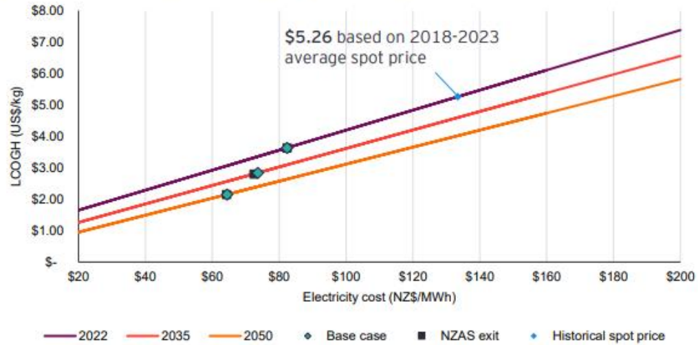
Figure 42: Electricity Input cost impact on Incremental centralised LCOGH
