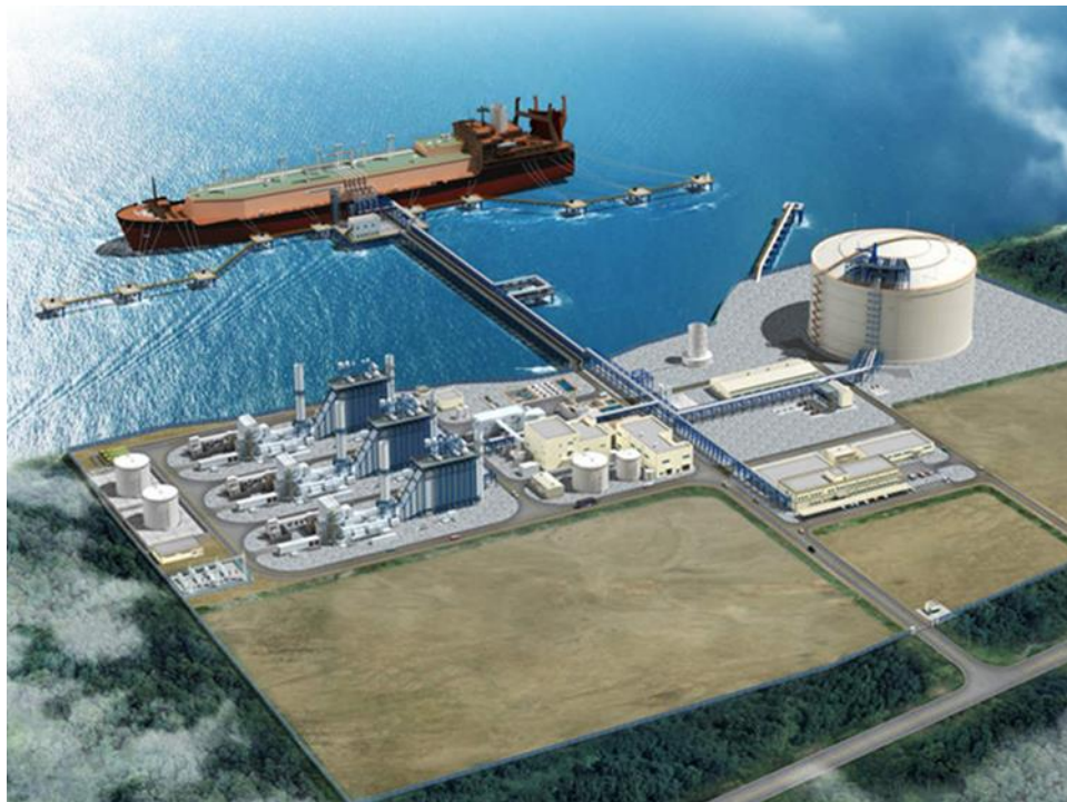
Figure 7-8: Port facility example, with LNG unloading, storage and power generation through 3 x CCGT units
