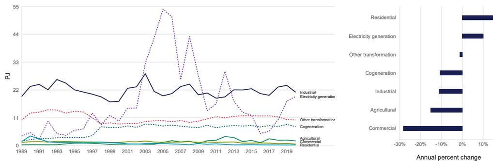
Coal use can be divided between consumption (which is further divided into Industrial, Agricultural, Commercial, and Residential consumption) and transformation (which is divided into Electricity Generation and Other Transformation). The total primary energy supply of coal (calculated as production and imports less losses and exports) for 2020 was 61 PJ, a decrease of 5.4 per cent on the previous year. Coal accounted for approximately 7.0 per cent of New Zealand's total consumer energy supply.
