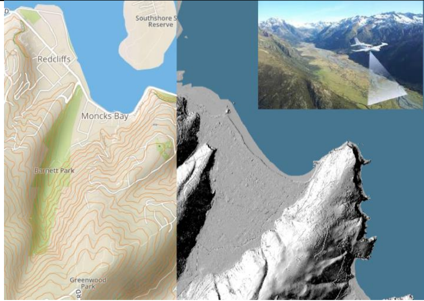
Figure 1 – LiDAR-based elevation data (right) provides a tenfold increase in accuracy compared to New Zealand’s current national dataset, which is based on topographic map contours. This improved accuracy is required for a number of applications, including evaluating flood risk or measuring slope when planning forestry operations.
