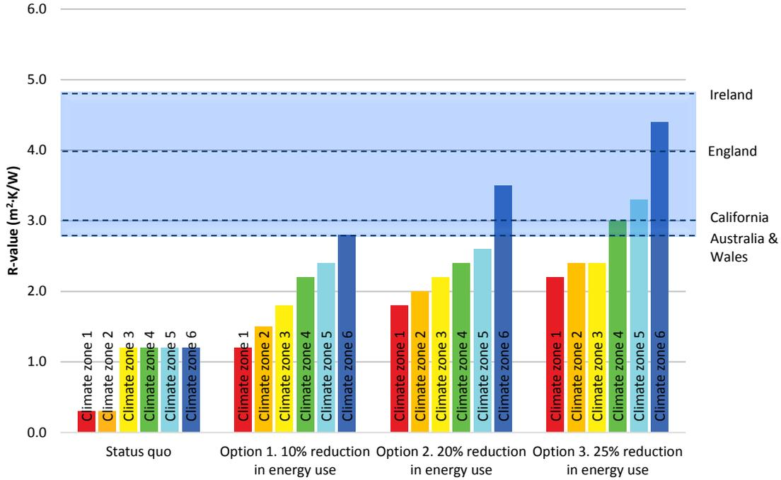
FIGURE 2.1D: Underfloor insulation – Proposed options compared to other parts of the world
