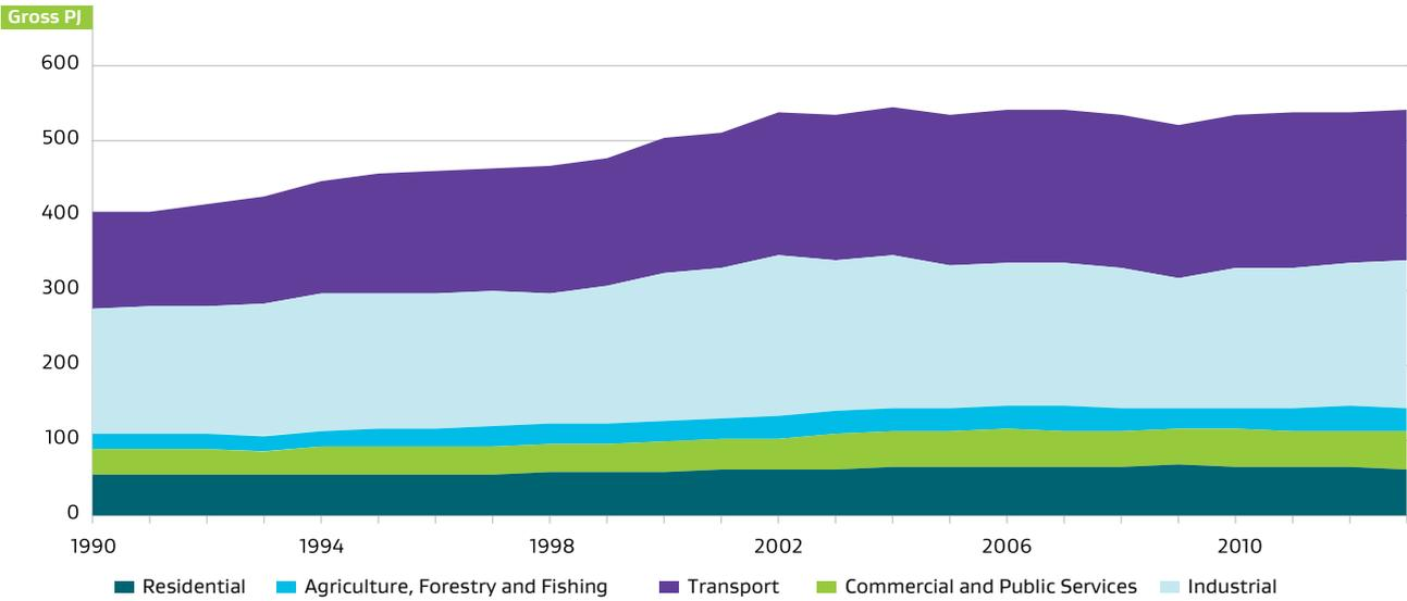
use by fuel since 1990. Non-energy use of gas peaked in 2000 when the Maui gas field was producing strongly.
