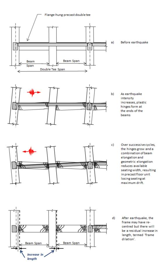
Figure 14: Illustration of beam elongation and frame dilation
