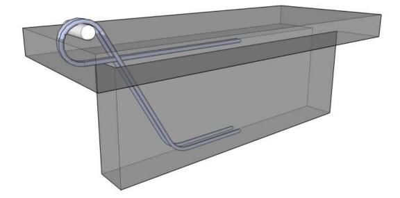
Figure 16: Loop bar hanger in precast double tee unit
