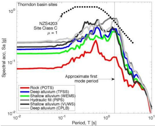
Figure 7: Geometric mean response spectra at strong motion stations located in Thorndon Basin relative to strong motion station on rock, for Sp=1
