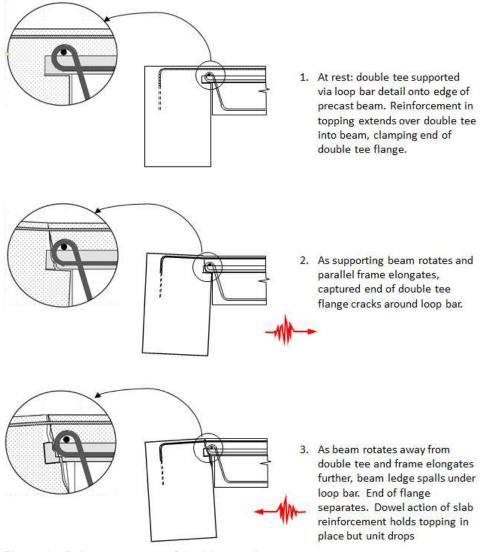
Figure 17: Failure sequence of double tee nib
