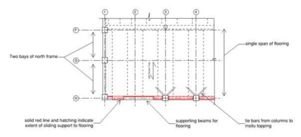
Figure 15: Part floor plan of northwest corner of typical floor showing two bays of beams per floor span
