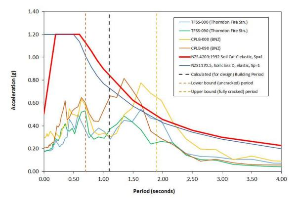
Figure 13: 5% damped acceleration response spectra at Thorndon Fire Station and BNZ Building strong motion stations
