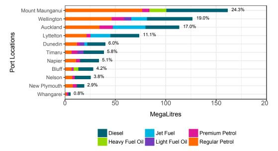
Fig 19 shows the net fuel capacities by type and terminal. Tank capacities include some volume of fuel at the bottom of a tank that is not generally accessible. Net fuel capacities subtract this volume from the overall volume of the tank.
