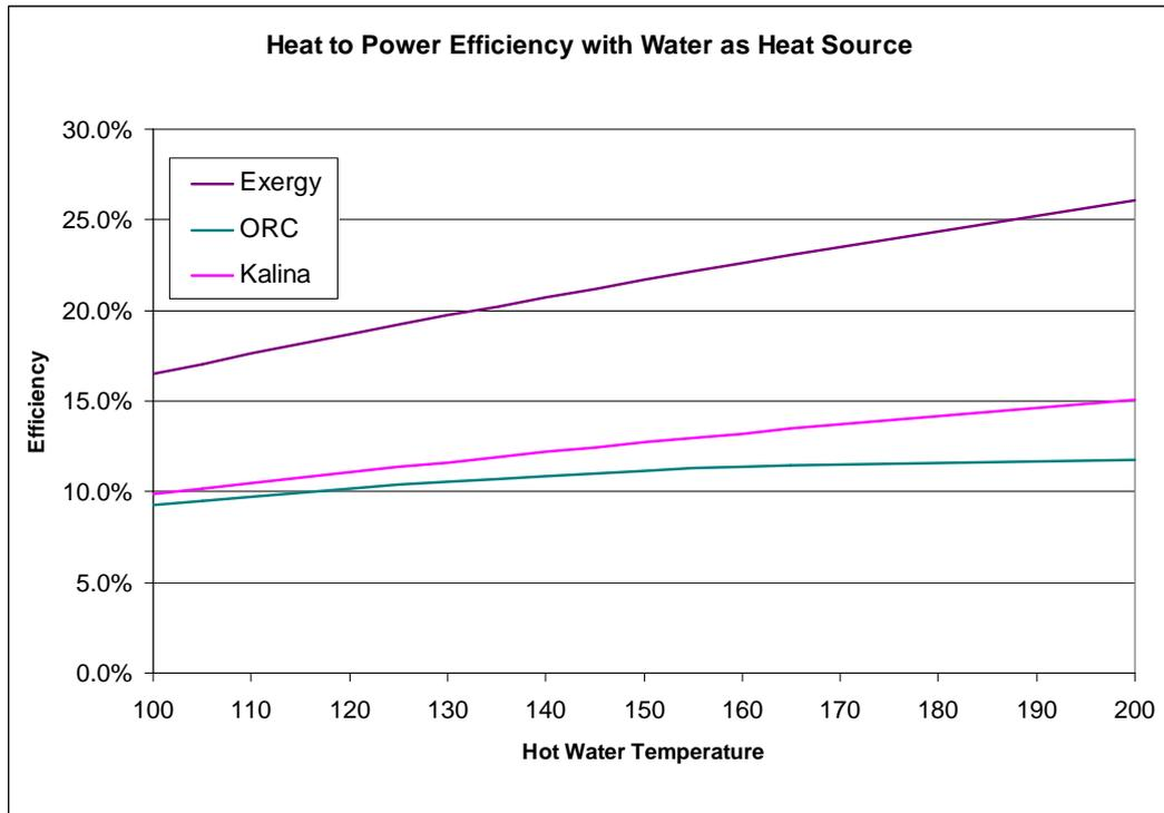
The exergy<sup>75</sup> line shown in this graph represents the absolute limit of mechanical work which is able to be extracted from the source heat according to the 2nd law of thermodynamics<sup>76</sup>. The proportion of the exergy actually converted to mechanical work is called the exergy efficiency and is a more meaningful reference for the performance of power conversion cycles at low temperatures than the energy efficiency.
