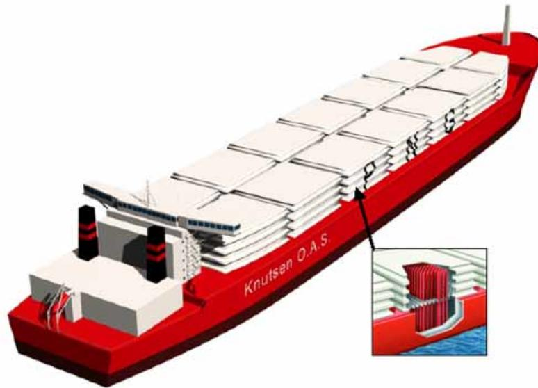
**Figure 6.2 - Transcanada barge mounted Gas Transport Modules (GTMs)**
