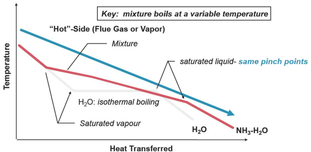
The Kalina cycle consists of a family of proprietary system designs that exploit the properties of the ammonia-water working fluid. Each design is applicable to a specific application, such as high temperature heat recovery (gas turbine based combined cycle) or geothermal brine. The families can consist of distillation/absorption/condensation subsystems, vapour generation/separation subsystems, or a combination of both.
