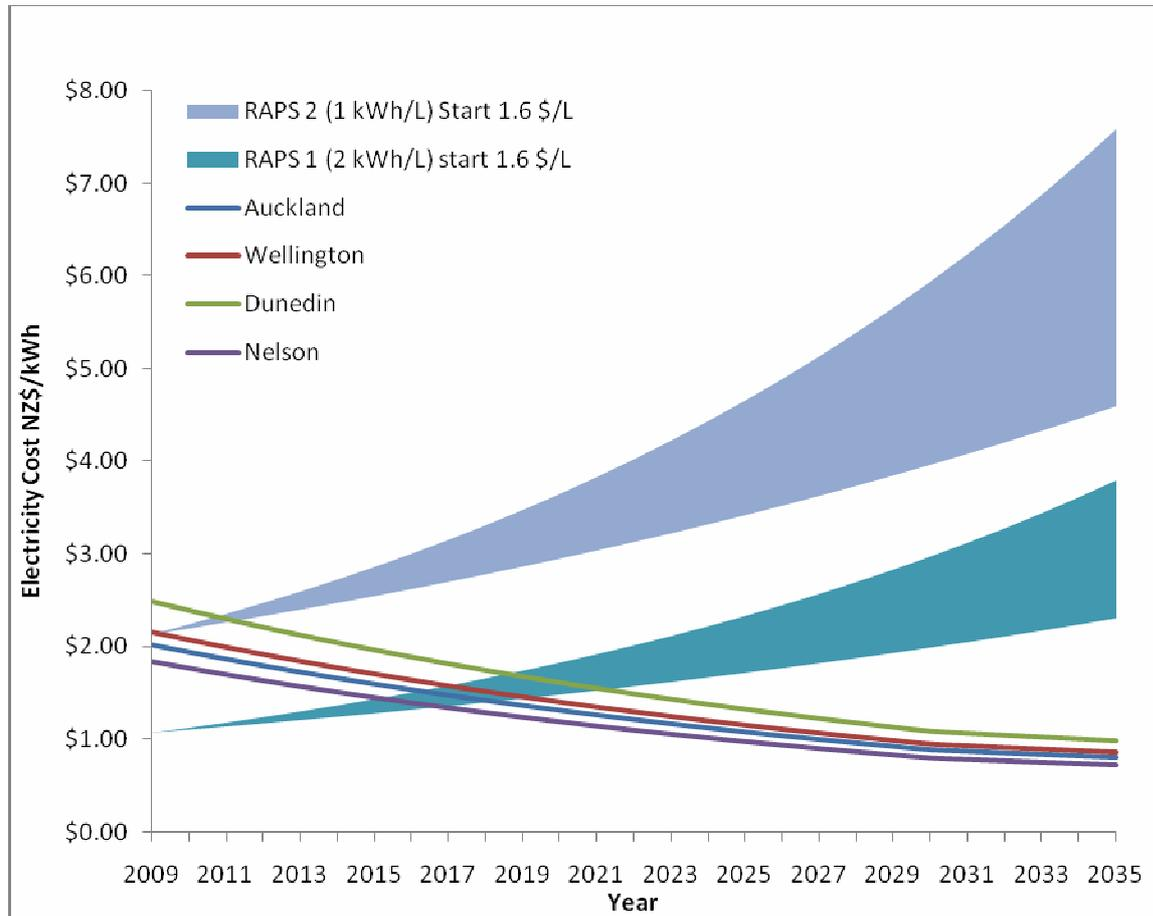
**Figure 8.4: Off-Grid PV Projections.** Projected electricity costs from PV based stand-alone power systems and 2 different diesel-based remote area power supply systems (RAPS) in different locations. The range of diesel price increases is between 3 and 5% per annum. For other assumptions, see Appendix 2.
